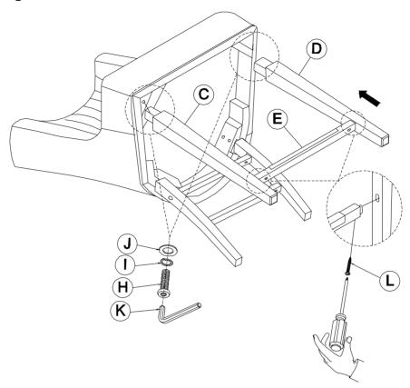
STEP 3: Using the Allen Key and Philips Head Screw driver to tighten the Bolts and screws
